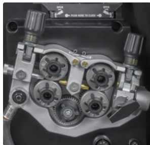
Heavy-duty aluminum four-drive-roll system.
