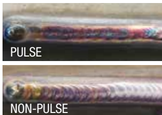
Example of Pulse vs Non-Pulse weld finish
