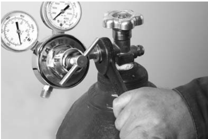
Figure 2. Attaching Oxygen Regulator
