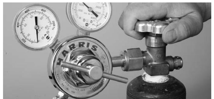
Figure 10. Opening Oxygen valve
