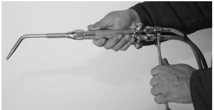
Figure 5. Attaching Hose to Torch
