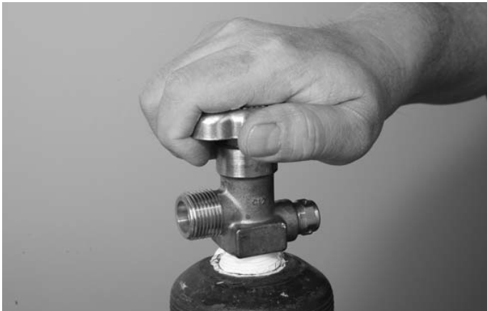
Figure 1. Opening Oxygen Cylinder Valve
