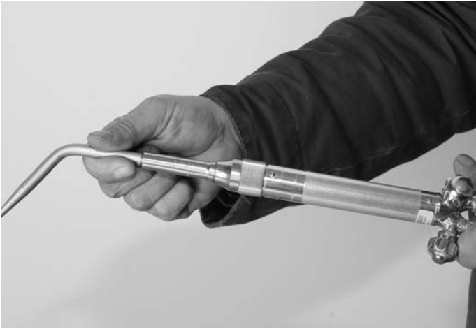
Figure 6. Installing Welding Tip
