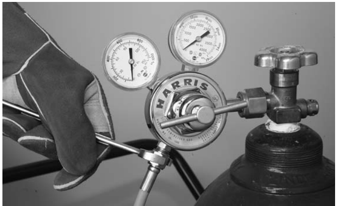
Figure 4. Attaching Hose to Regulator
