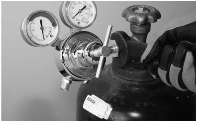
Figure 3. Attaching Fuel Gas Regulator
