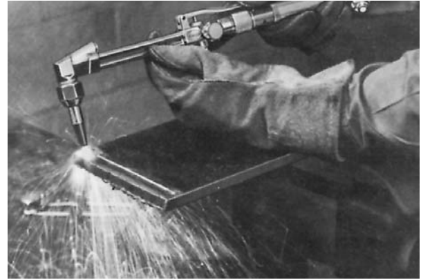
Figure 19. Steel Flame Cutting
