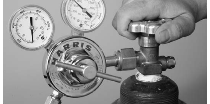
Figure 9. Opening Fuel Gas Cylinder Valve
