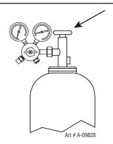
Figure 3-9: Open Cylinder Valve
