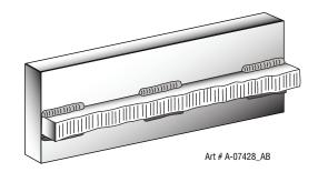
Figure 4-26: Chain Intermittent Welding
