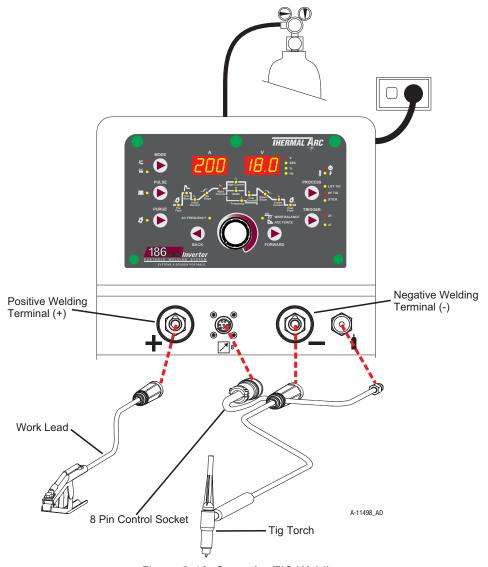
Figure 3-10: Setup for TIG Welding
