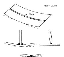
Figure 4-23: Examples of Distortion
