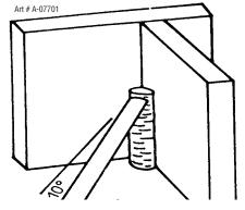
Figure 4-15: Single Run Vertical Fillet Weld
