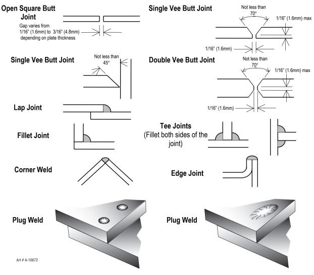
Figure 4-9: Typical Joint Designs for Arc Welding
