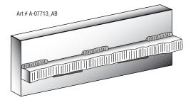
Figure 4-27: Staggered Intermittent Welding
