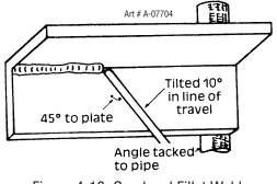
Figure 4-18: Overhead Fillet Weld
