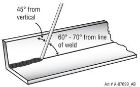
Figure 4-13: Electrode Position for HV Fillet Weld
