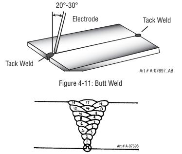
Figure 4-12: Weld Build up Sequence
