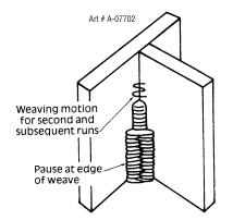
Figure 4-16: Multi Run Vertical Fillet Weld
