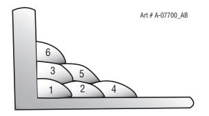
Figure 4-`14: Multi-runs in HV Fillet Weld
