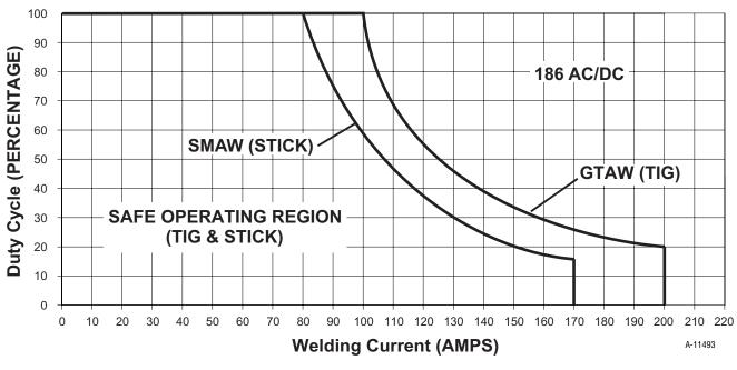
Figure 2-2: 186 AC/DC Duty Cycle
