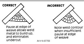
Figure 4-17: Examples of Vertical Fillet Welds
