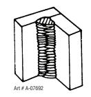
Figure 4-6: Vertical Position, Fillet Weld
