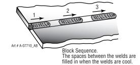
Figure 4-24: Welding Sequence
