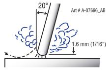
Figure 4-10: Striking an Arc
