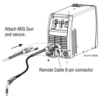
Figure 3-8: Mount MIG Gun Cable to Adapter Socket
