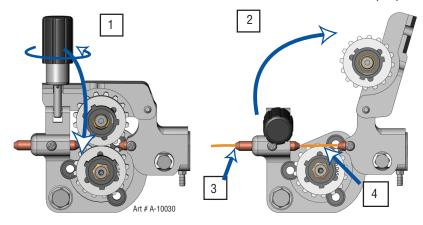
Figure 3-11: Opening Pressure Arm and Inserting Wire
