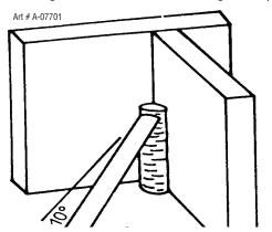
Figure 4-25: Single Run Vertical Fillet Weld
