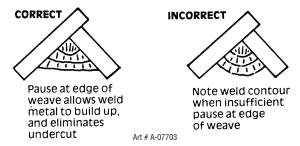
Figure 4-27: Examples of Vertical Fillet Welds
