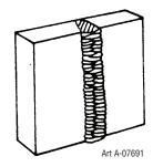
Figure 4-15: Vertical Position, Butt Weld
