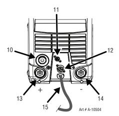
Figure 3-2: Fabricator Front Connections
