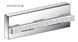
Figure 4-37: Staggered Intermittent Welding
