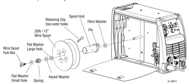
Figure 3-10: Standard 33 lb 12" Spool Installation
