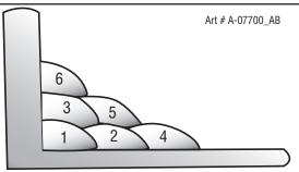
Figure 4-24: Multi-runs in HV Fillet Weld
