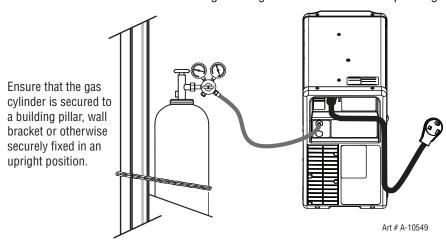
Figure 3-18: Attach gas line to proper inlet
