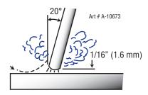
Figure 4-20: Striking an Arc
