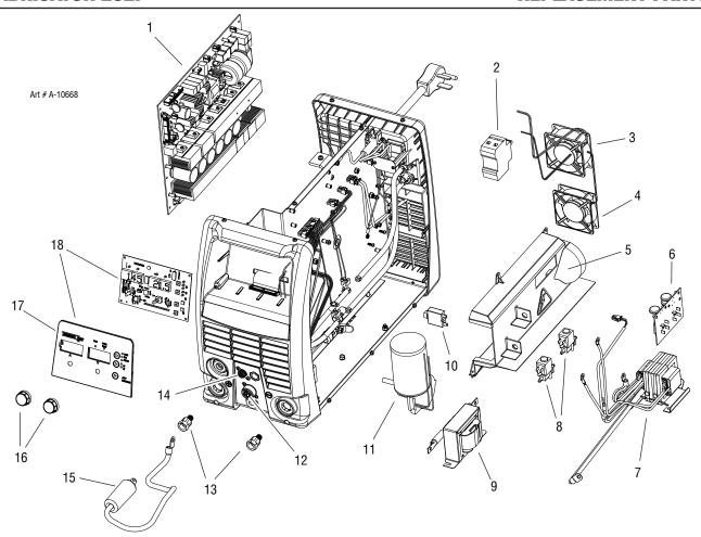
Figure 6-4: Right side and Front Replacement Parts
