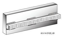
Figure 4-36: Chain Intermittent Welding
