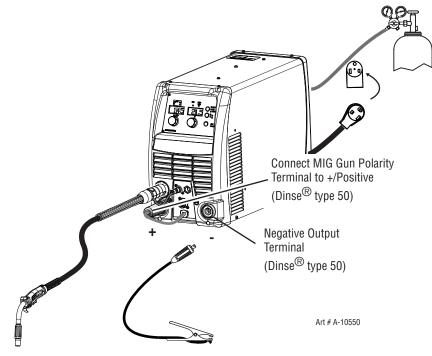
Ensure that the gas cylinder is secured to a building pillar, wall bracket or otherwise securely fixed in an upright position.
