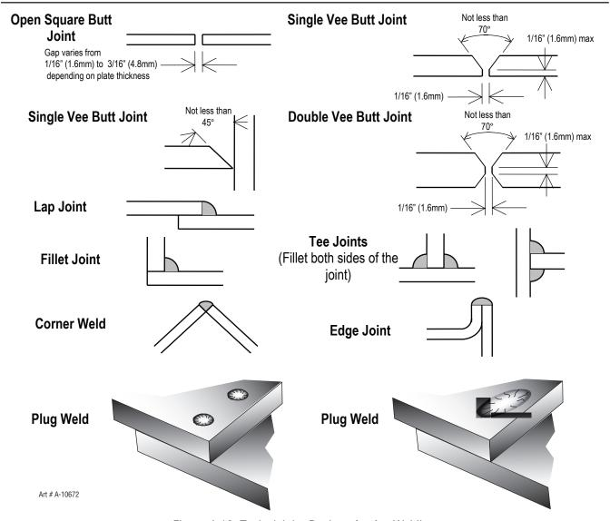
Figure 4-19: Typical Joint Designs for Arc Welding
