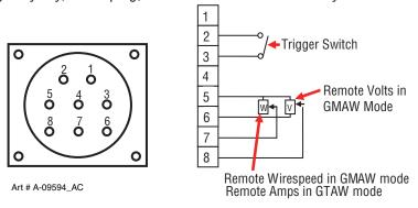
Figure 3-3: Remote Control Socket
