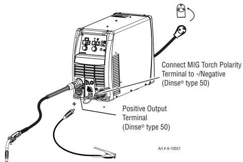
Figure 3-21: MIG Gun Polarity Negative
