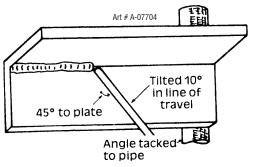
Figure 4-28: Overhead Fillet Weld
