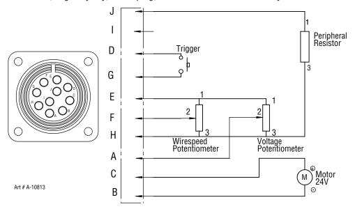
Figure 3-4: Remote Control Socket
