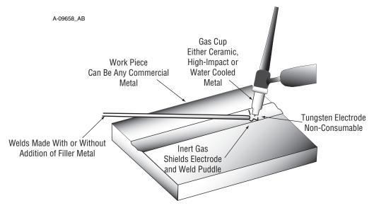
Figure 4-6: TIG (GTAW) Welding Application Shot
