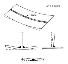
Figure 4-33: Examples of Distortion
