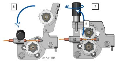
Figure 3-12: Closing Pressure Arm and Adjusting Tension
