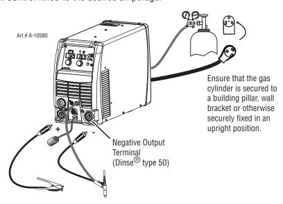
Figure 3-23: Setup for LIFT TIG (GTAW) Welding
