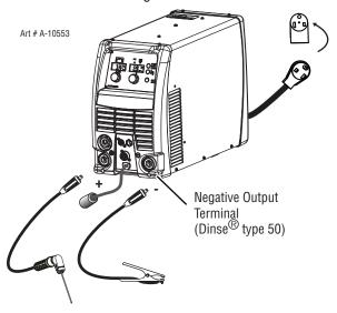
Figure 3-24: Setup for STICK Welding reverse polarity shown.
