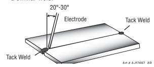
Figure 4-21: Butt Weld
