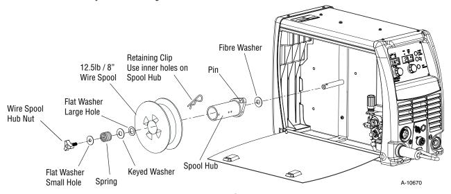
Figure 3-9: 12.5 lb 8" Spool Installation
