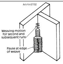
Figure 4-26: Multi Run Vertical Fillet Weld
