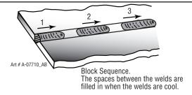
Figure 4-34: Welding Sequence
