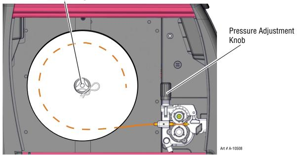
Figure 3-16: Wire Installed
