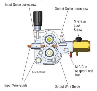
Figure 3-15: Wire Guide Installation
