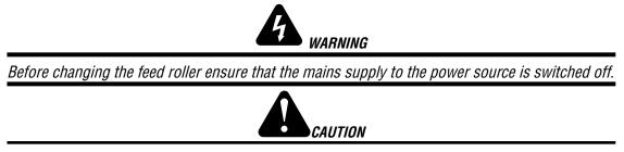
The use of excessive pressure may cause rapid wear of the feed rollers, shafts and bearing.
